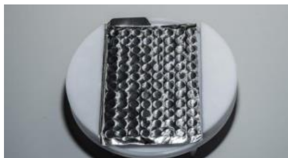
Figure 3: Sealing the DiaEasy™ Dialyzer tubes in 96-well format with the included aluminum foil adhesive sealer. Ensure that the rim of each tube is in contact with the sealer.
