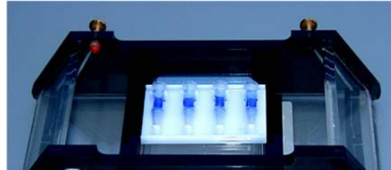
Figure 3: Supporting tray containing three DiaEasy™ Dialyzer tubes in a horizontal electrophoresis tank. The arrow on the cap is positioned face up and the two membranes of the DiaEasy™ Dialyzer tubes are in perpendicular to the electric field.
