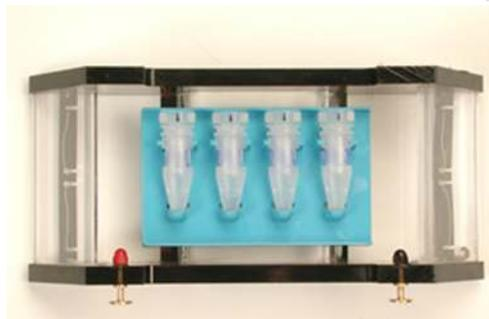
**Figure 2:** Supporting tray containing three DiaEasy™ Dialyzer tubes in a horizontal electrophoresis tank. The arrow on the cap is positioned face up and the two membranes of the DiaEasy™ Dialyzer tubes are in perpendicular to the electric field.
