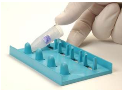
Figure 1: Insertion of the DiaEasy™ Dialyzer tubes in the provided supporting tray. The arrow on the cap is positioned face-up.
