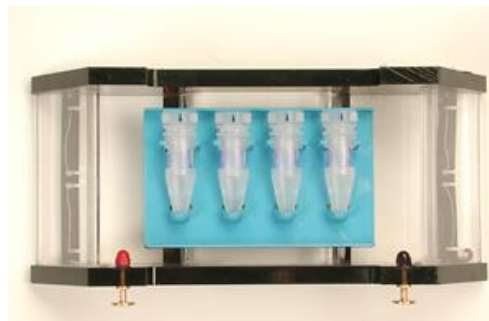
Figure 2: Supporting tray containing three DiaEasy™ Dialyzer tubes in a horizontal electrophoresis tank. The arrow on the cap is positioned face up and the two membranes of the DiaEasy™ Dialyzer tubes are in perpendicular to the electric field.
