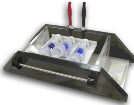
Figure 3: Supporting tray containing three DiaEasy™ Dialyzer tubes in a horizontal electrophoresis tank. The arrow on the cap is positioned face up and the two membranes of the DiaEasy™ Dialyzer tubes are in perpendicular to the electric field.
