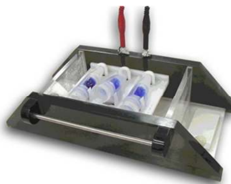
Figure 2: Supporting tray containing three DiaEasy™ Dialyzer tubes in a horizontal electrophoresis tank. The arrow on the cap is positioned face up and the two membranes of the DiaEasy™ Dialyzer tubes are in perpendicular to the electric field.
