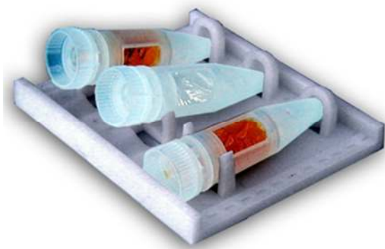
Figure 1: Insertion of the DiaEasy™ Dialyzer tubes in the provided supporting tray. The arrow on the cap is positioned face-up.
