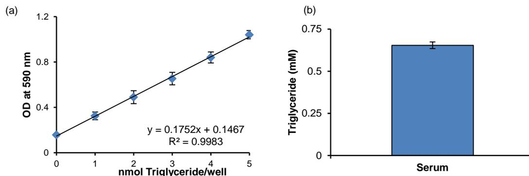
**Figure:** (a) Triglyceride Standard Curve. (b) Determination of Triglyceride in pooled normal human serum. Undiluted serum sample (2  $\mu$ l) was assayed directly (no prior treatment) according to the kit protocol. Calculated concentration of triglyceride:  $0.65 \pm 0.02$  mM; ( $58 \pm 1.8$  mg/dl).
